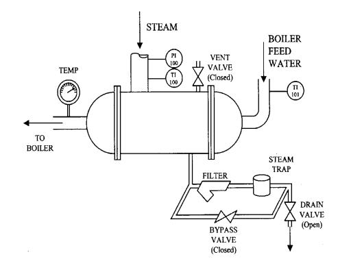
Waste flash steam from the ethyl acetate plant is saturated at slightly above atmospheric pressure. It is sent to the shell of a shell and tube heat exchanger to preheat the boiler feed water to 70°C for the nearby boiler house.
