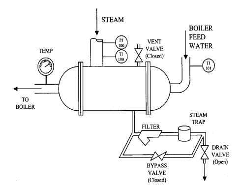
Condensate is withdrawn through a thermodynamic steam trap at the bottom of the shell. The water flows once through the 3/4" nominal tubes. There are 1000 tubes. "When the system was put into operation 3 hours ago everything worked fine," says the supervisor. "Now, however, the exit boiler feed water is 42°C instead of the design value. What do we do? This difficulty is costing us extra fuel to vaporize the water at the boiler." Fix it. • What are the fundamentals of heat exchange?
